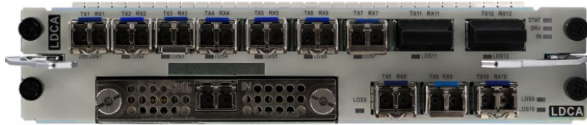
Figure 2: Huawei LDCA Board
