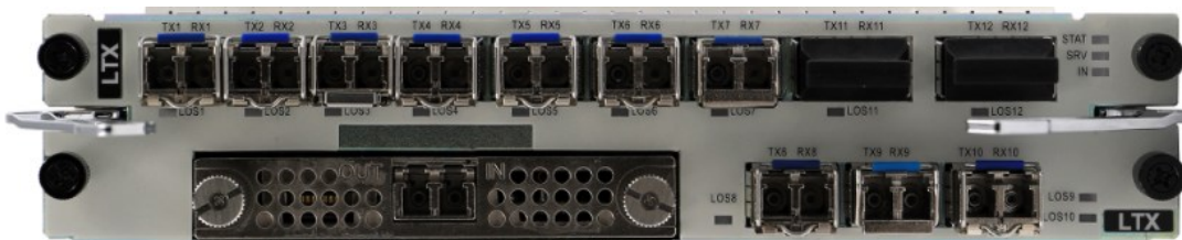
Figure 5: Huawei LTX Board
