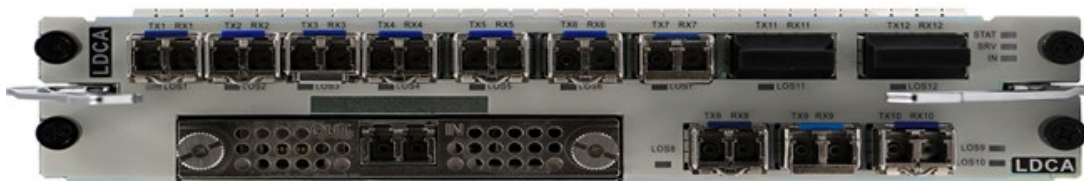
Figure 3: Huawei LDCA Board
