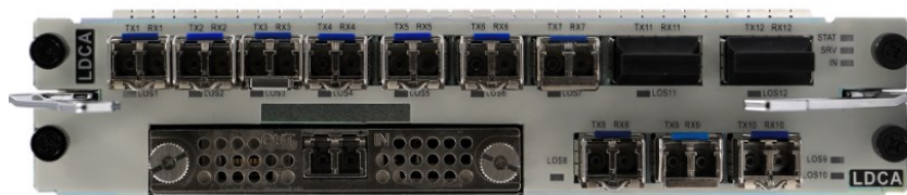
Figure 2: Huawei LDCA Board
