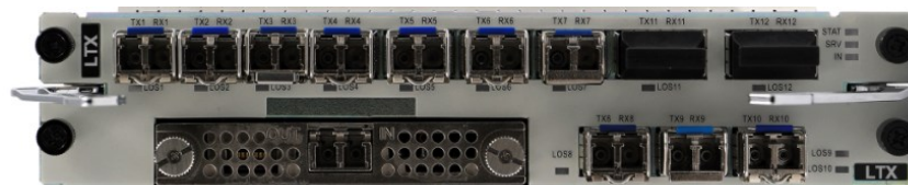
Figure 3: Huawei LTX Board
