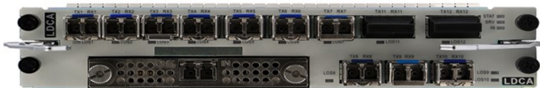
Figure 3: Huawei LDCA Board
