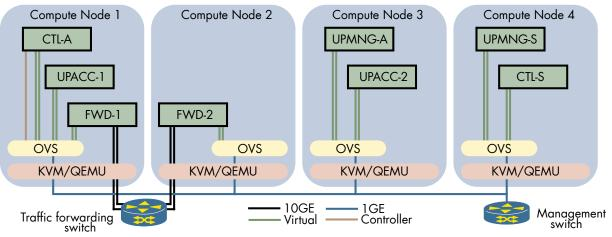
Figure 1: Network Cloud Engine
